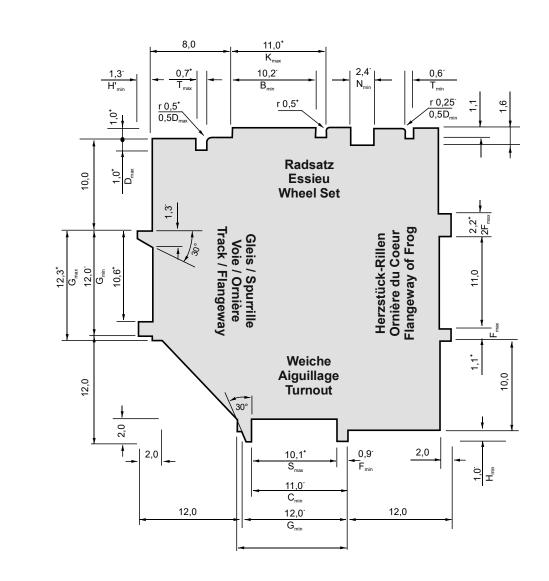
Guide tolerances: + means +0.03 - 0 - means +0 - 0.03 Clearance tolerance 0.5
